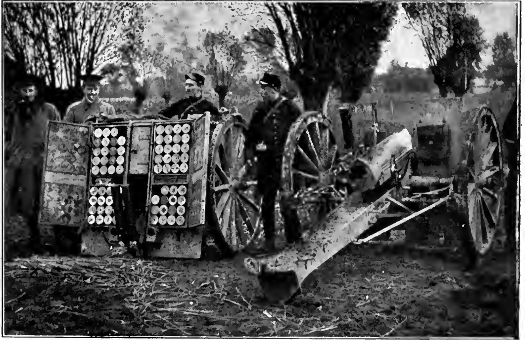
A FRENCH 75-MM. GUN, SHOWING BREECH MECHANISM AND AMMUNITION LIMBER.
